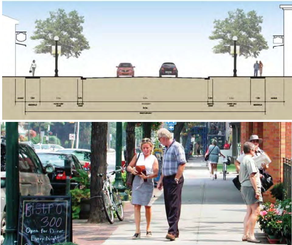
Figure X5.13: Alternative 3 (Long-term) - As part of the reconstruction of the Guelph Street right-of-way (in combination with the Norval interchange), a wider right-of-way width could allow the proper boulevard width to accommodate street trees, lighting and banners, and pedestrian amenities on both sides.
