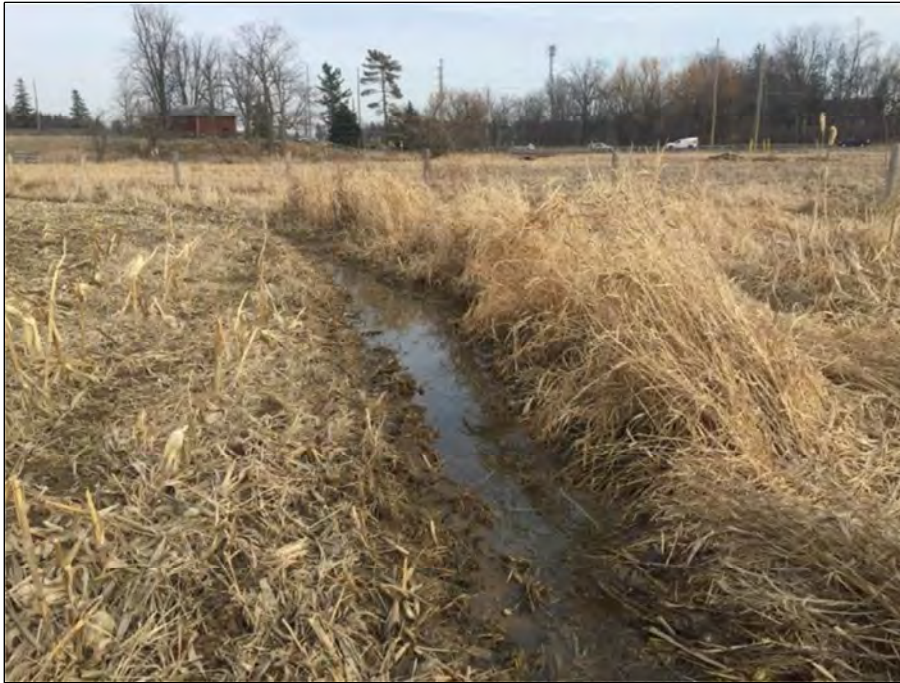
126. HDF -1 (Segment 2). Facing downstream, flow path is more defined. Feature type is swale and flow condition is surface flow minimal. Wetted depth is 18 cm.
