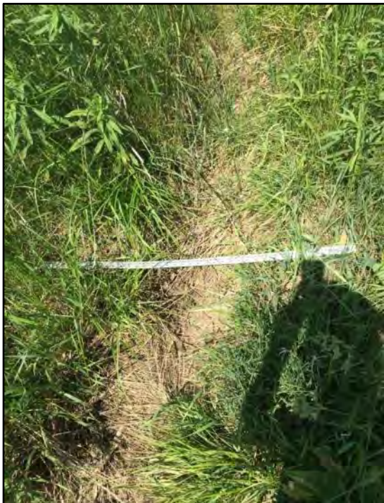
89. HT-2b-3 Depression is approximately 0.5m in width and 0.15m in depth.
