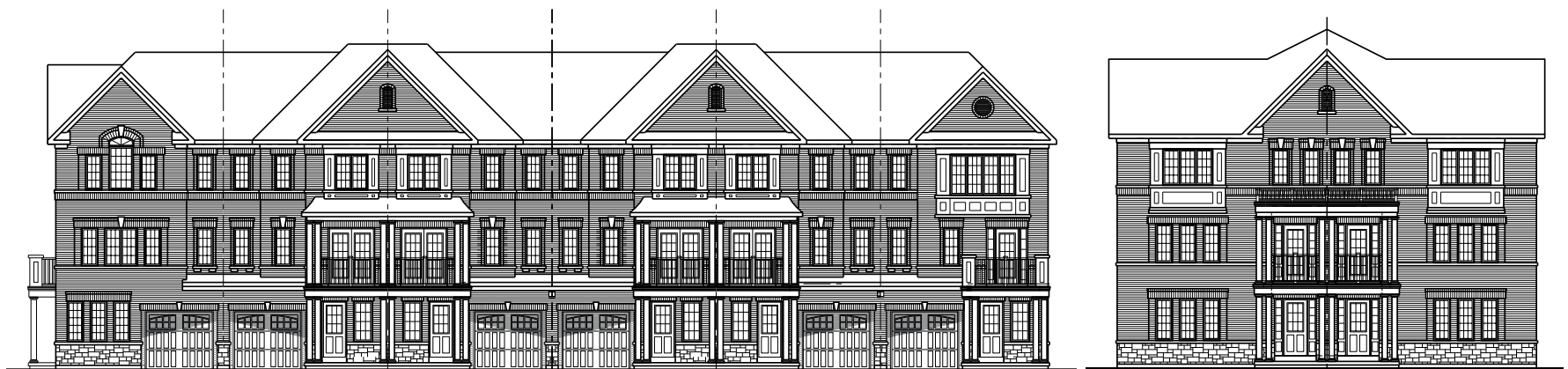
FRONT / REAR ELEVATIONS
