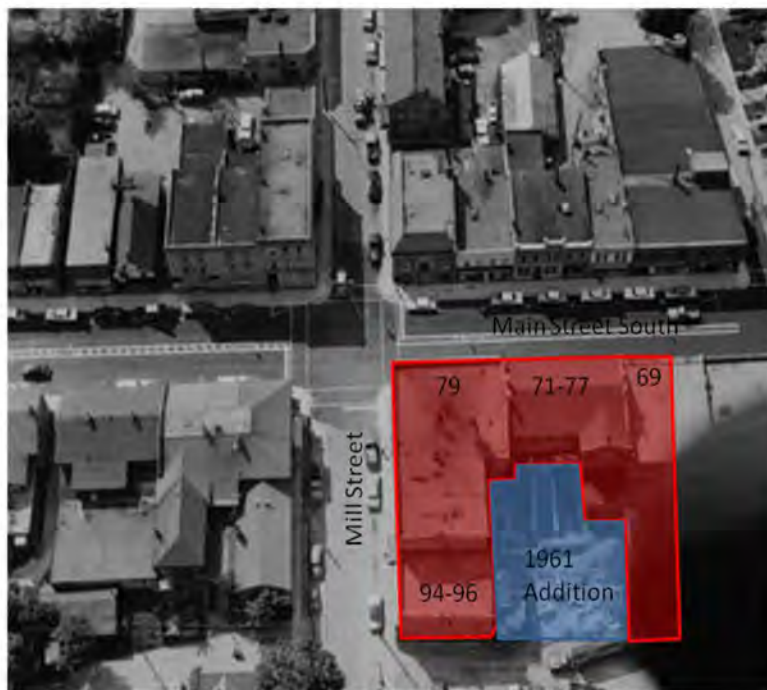
Figure 22: 1961 Aerial Photograph showing approximate boundaries of buildings in the study area and boundaries of the 1961 addition, then under construction (Adapted from a Silvercreek Commercial Builders PowerPoint Presentation to Heritage Halton Hills, April 2014).
