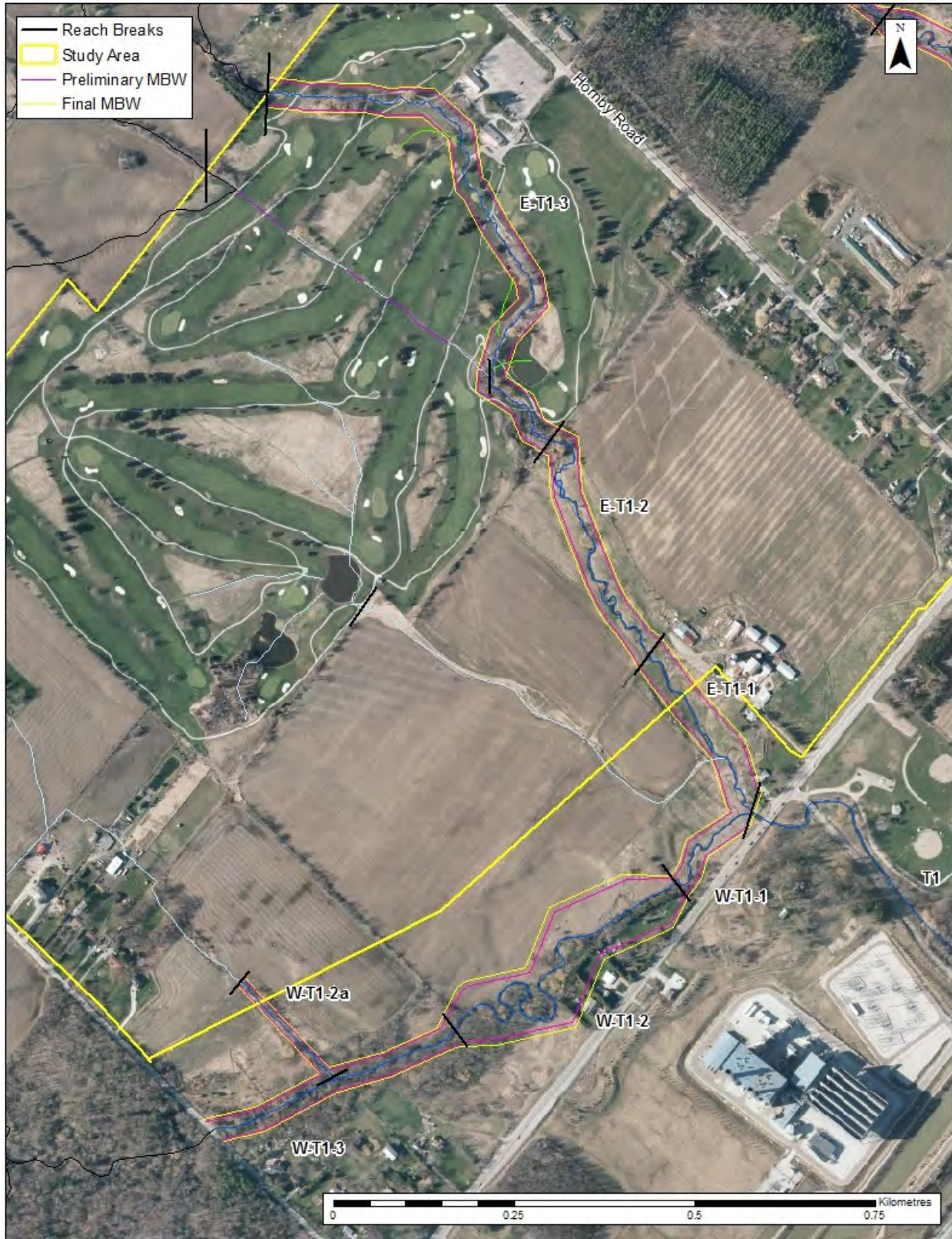
FIGURE D-1-2 Meander belt delineation for Middle Sixteen Mile Creek Tributary reaches
