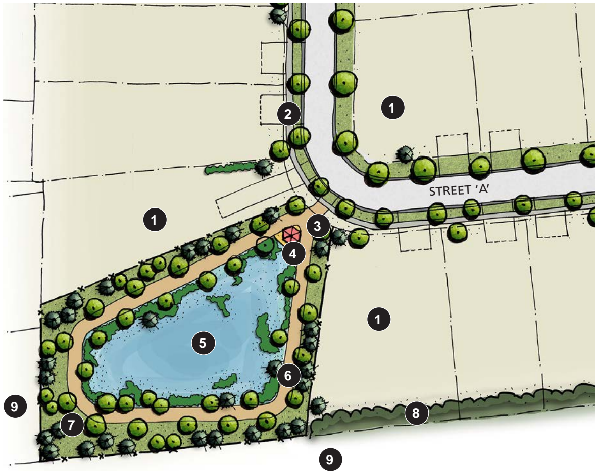
Figure 17: Conceptual Stormwater Management Pond Design.
