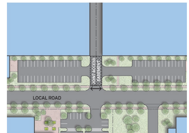
Recommended Driveway with Joint Access Easement
