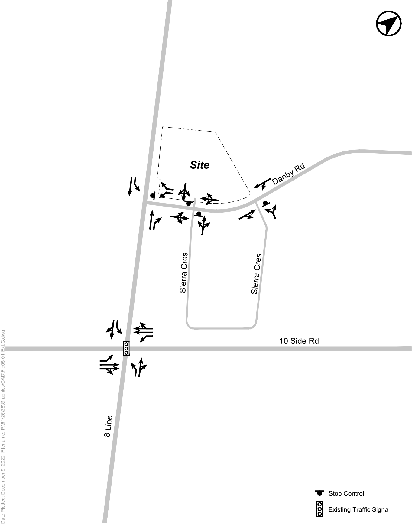
FIGURE 5 EXISTING LANE CONFIGURATION AND TRAFFIC CONTROL
