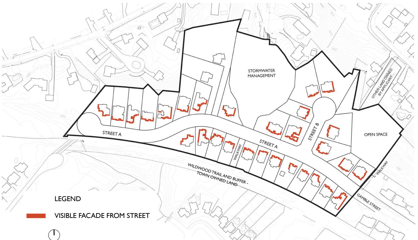
Figure 8 - Streetscape Elevation Relationship Diagram
