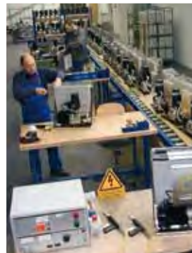
Assembly line for rainwater units.
