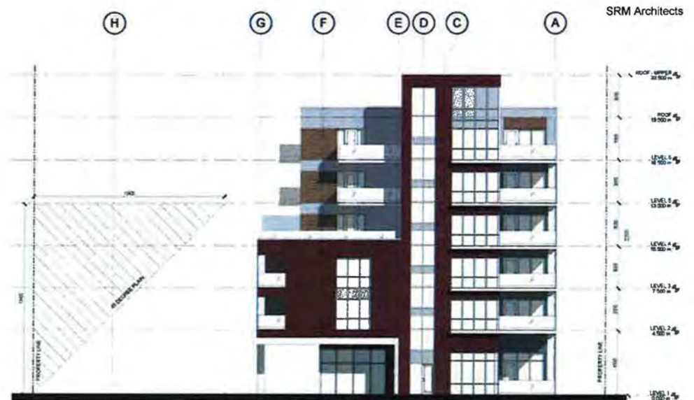
Figure 20 – Project East Elevation
