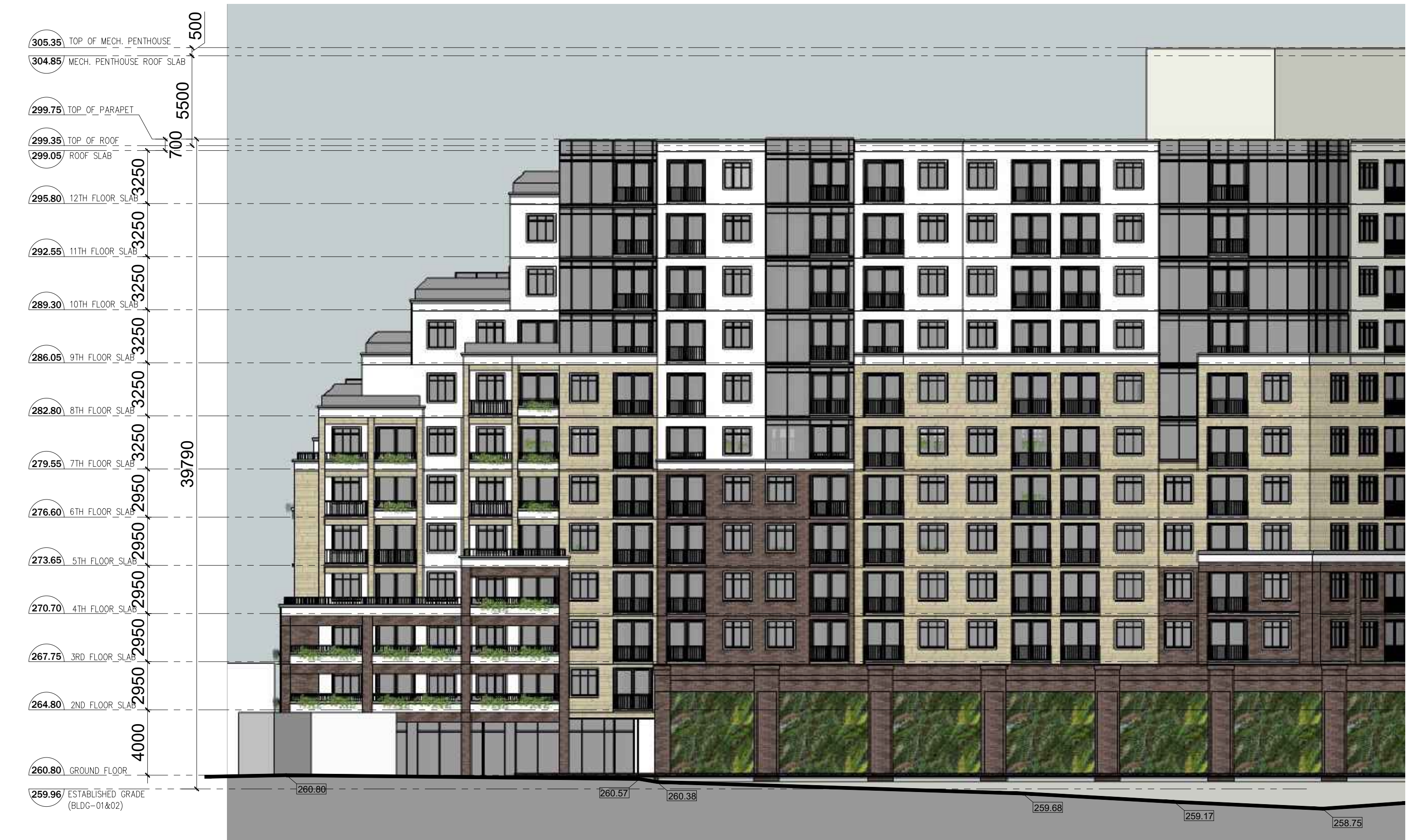
BUILDING - 2 _ WEST ELEVATION _ SCALE 1:200
