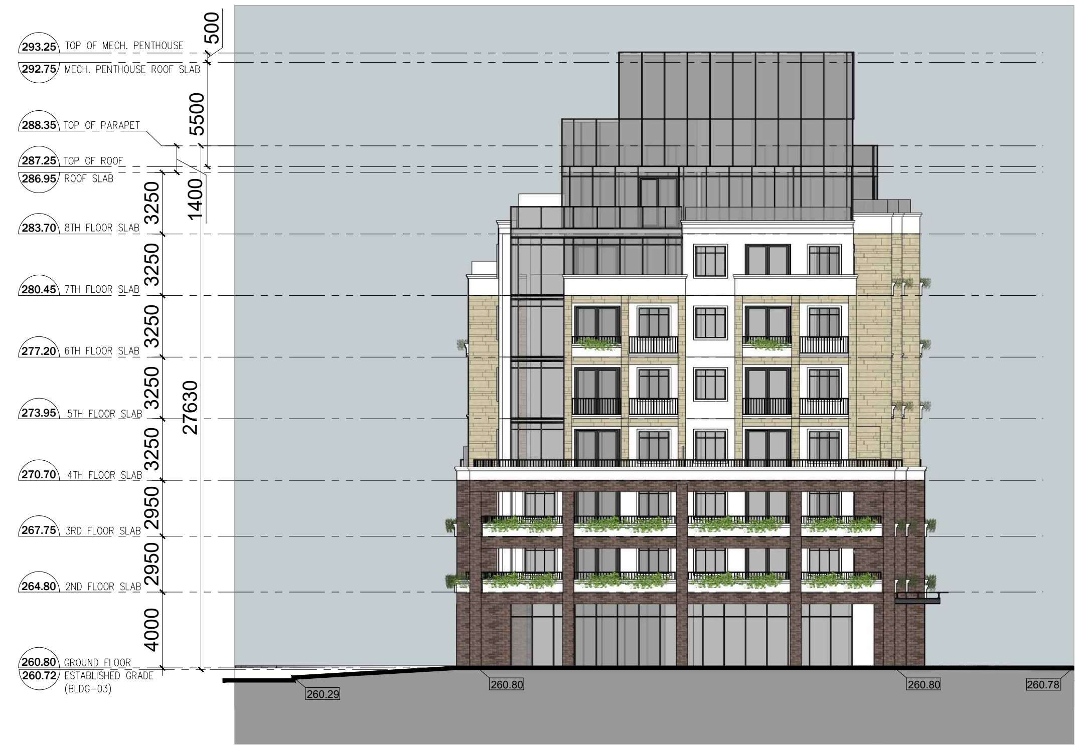
BUILDING - 3 _ NORTH ELEVATION _ SCALE 1:200
