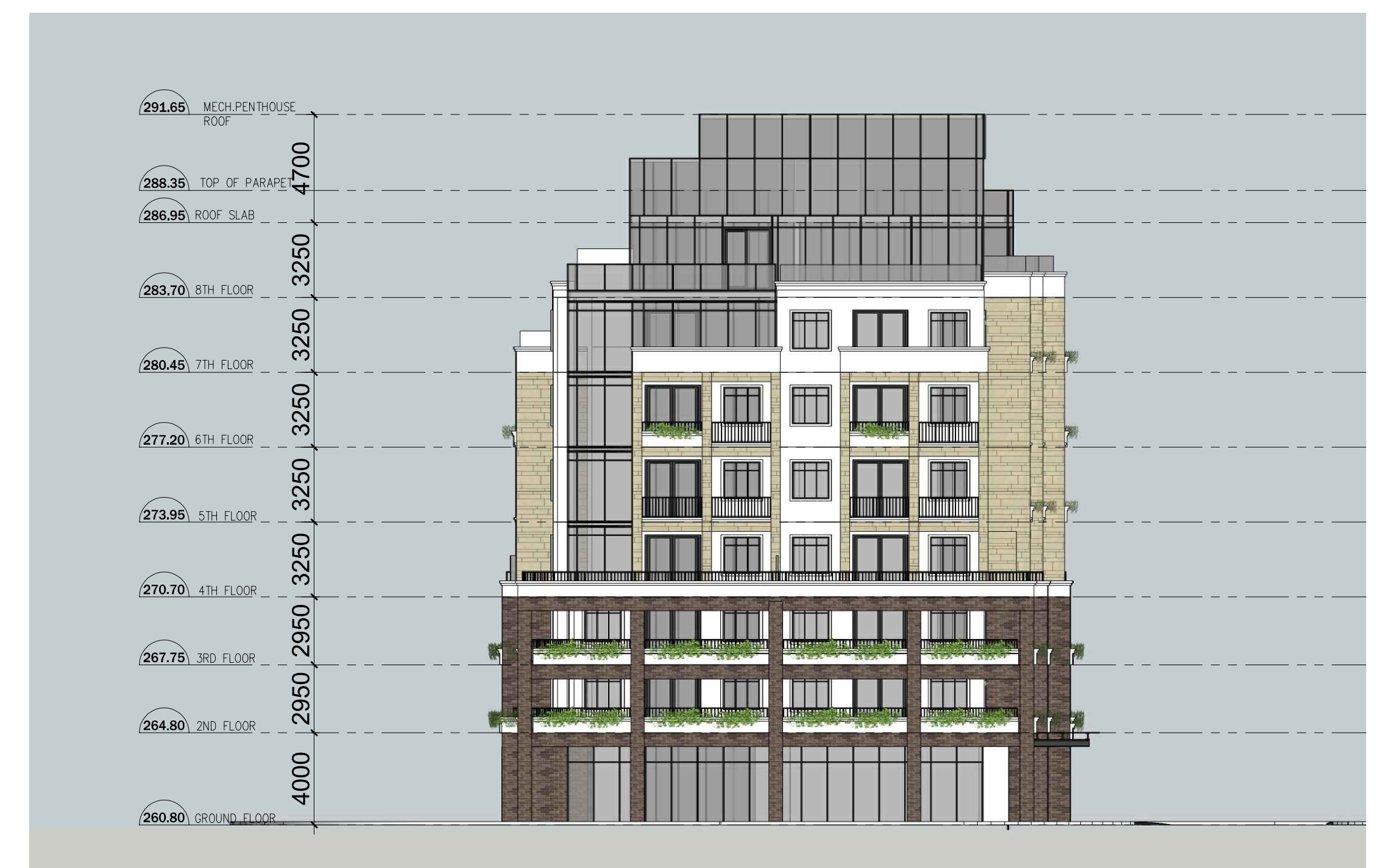
BUILDING - 3 _ NORTH ELEVATION _ SCALE 1:200
