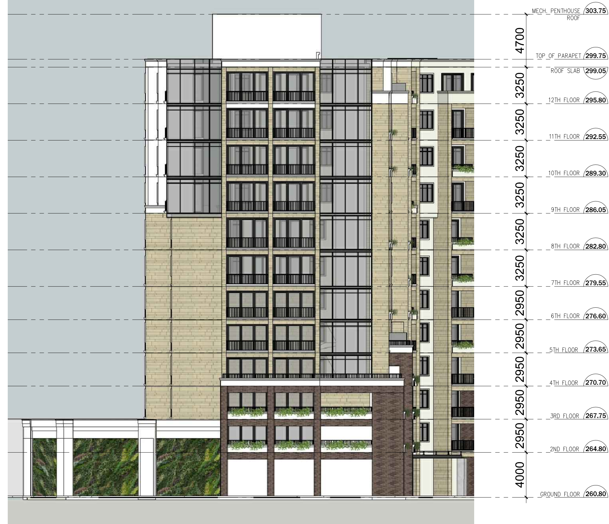
BUILDING - 1 _ EAST ELEVATION _ SCALE 1:200
