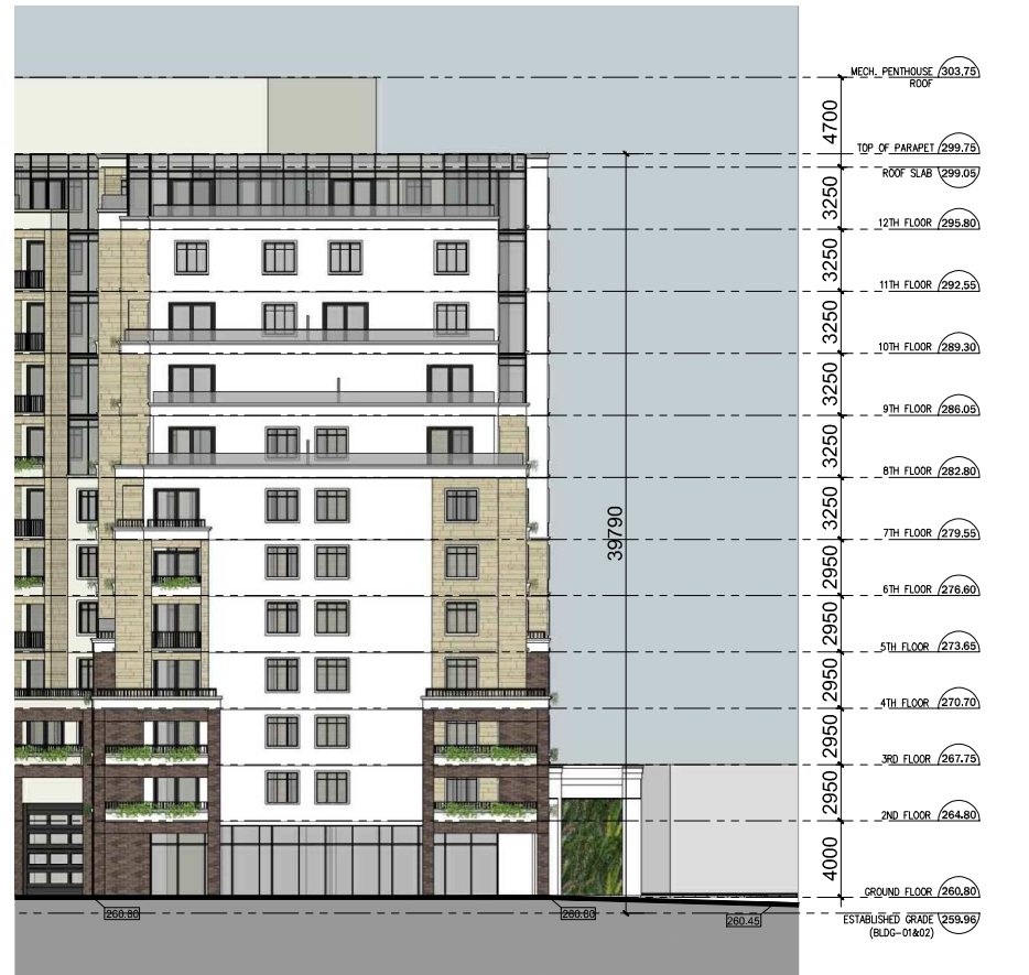
BUILDING - 2 _ NORTH ELEVATION _ SCALE 1:200
