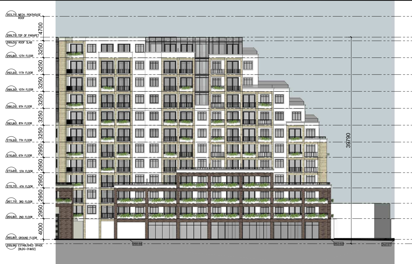
BUILDING - 2 _ EAST ELEVATION _ SCALE 1:200
